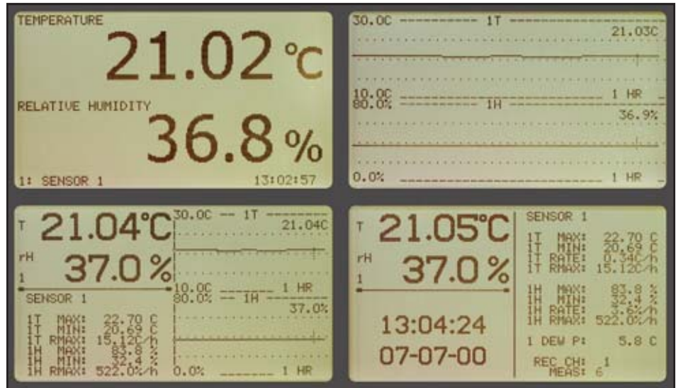
The DewK lets you view data just about any way you like it. Both graphical data and statistical data can be shown for temperature and humidity from one or two inputs. Modifying any of the standard screens is easily done, so you see exactly what you want—no more, no less.
